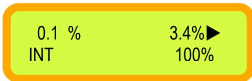
When you first power up the LM5, the display will briefly show the product version. Then the following; Desired grade selection (top left) Real-time grade (top right) Internal vial (INT) or External Sensor (EXT) and battery percentage (if internal battery is being used)
