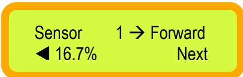
This menu allows for orientation of the sensor in regards to the machines forward travel. When using an external sensor enter the number on the top of the sensor which is pointing in the forward travel of the machine. For internal sensors the configuration should be set to 1 - Forward. The menu defaults back to main screen after 15 seconds.
