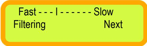
The LM-5 is designed with a fast response time. This fast response also reflects machine acceleration. Either vibrations or accelerations can cause erratic grade control. To reduce these false signals, it will be necessary to 'slow down' the sensor to some degree. Select the fastest filtering level that produces stable machine control.
