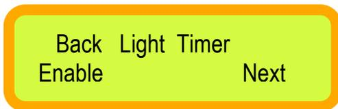
The first menu item is for selecting the backlight configuration. Select the Flip button to enable or disable the backlight option. \*Note: Battery life for time enabled is rated for 200 hours and disabled 12 hours of battery life. Select Next for following menu
