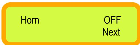
Using either arrow keys you can turn the Horn option on or off. Select Next for following menu
