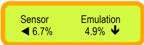
The left number value shows the left/right slope to 0 grade ratio and the right value displays front/back percentage. This screen verifies that the vial has valid readings in regards to its zero position
