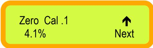
This screen is required to calibrate the LM5 to the terrain slope your equipment is situated on. This is described further under the calibration part of the manual.
