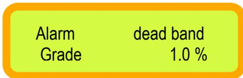
If horn is enabled the dead band grade settings can be changed. Alarm will sound when you go past the dialed in grade plus this offset. (ex. If grade setting is set at 0% and dead band is set at 1.0% the alarm will sound at any grade +1% and at any grade less than -1% slope)
