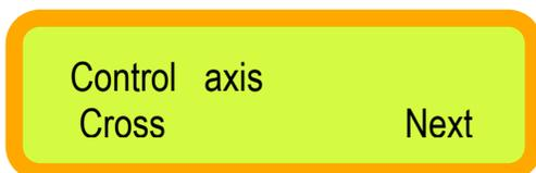
This menu allows the user to indicate which sensor orientation to use for their machine. There is 2 options either Cross rotation (left and right) or Fwd/Back (front and back).
