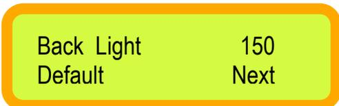
This screen allows for backlight brightness. Select up or down arrows to change. Select Default for factory setting. This screen will change back to main menu after 15 second.
